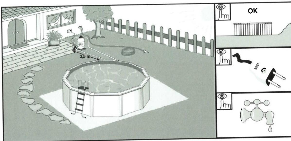
**EN** **Installation place:** Our pools are designed to be erected above ground and for an outdoor family use. The ground has to be firm, flat and perfectly horizontal. **Remember:** 1000 lts of water =  $1 \text{ m}^3 = 1000 \text{ Kgs}$ .
