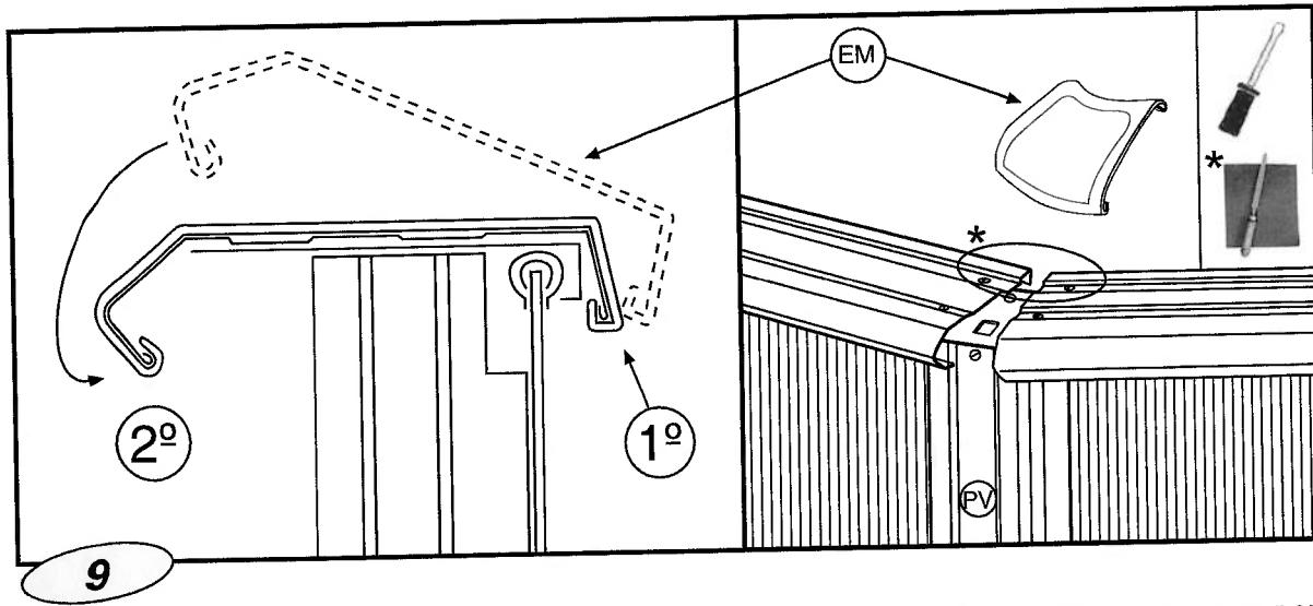
**EN** \* **IMPORTANT! BEFORE ASSEMBLY, DEBURRING, USING A FILE AND SANDPAPER, THE ENDS OF EACH EDGE.**
